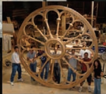
New wood frame, stained glass conservation/restoration and storm glass for St. Luke Episcopal Church, Racine, WI
