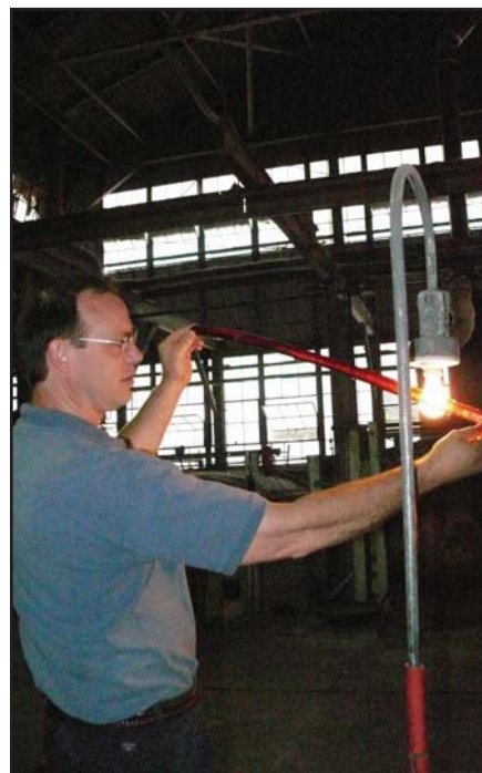
Mark Feldmeier checks stringers of glass for correct color.
