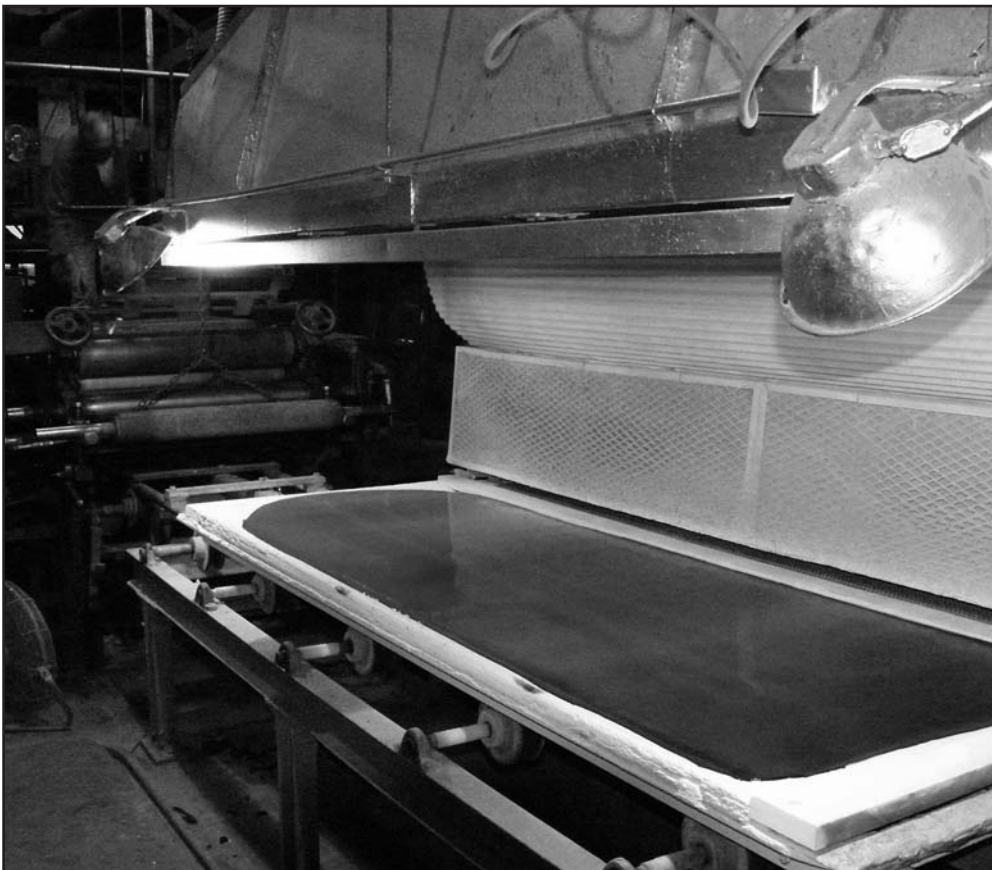
The glass is rolled into a sheet and then is sent into the anneal lehr to cool.
